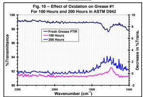
On the <u>right-hand</u> ordinate, the FTIR values of Percent Transmittance for the <u>oxidized</u> grease samples are subtracted from those of the <u>fresh</u> grease (in this case Grease #1). This shows the effects of oxidation on the fresh test grease by the increase in concentration of oxidized grease components and thus a decrease in Percent Transmittance.
