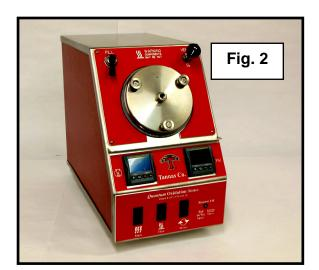
The design of the bath-free Quantum also permits access to the test substance in the pressure chamber during test to extract a small sample [7].
