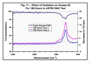
The peaks of Test 1 and Test 2 are both at 1710 cm<sup>-1</sup> with reduced Percent Transmittance of 17% and 11% respectively at this wavenumber closely associated with hydrocarbon oxidation.
