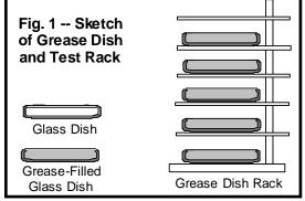
The combined stack of grease-filled dishes are then inserted into a cylindrical pressure chamber and exposed to oxygen of not less than 99.5% purity at an initial pressure of 100 pounds per square inch (PSI = 690 kPa) and room temperature which is then increased to 99  $\pm 0.5^{\circ}$ C. Under this increased temperature, the oxygen pressure is carefully released to maintain no more than 110  $\pm 2$  PSI).
