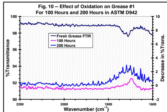
On the right-hand ordinate, the FTIR values of Percent Transmittance for the oxidized grease samples are subtracted from those of the fresh grease (in this case Grease #1). This shows the effects of oxidation on the fresh test grease by the increase in concentration of oxidized grease components and thus a decrease in Percent Transmittance.
