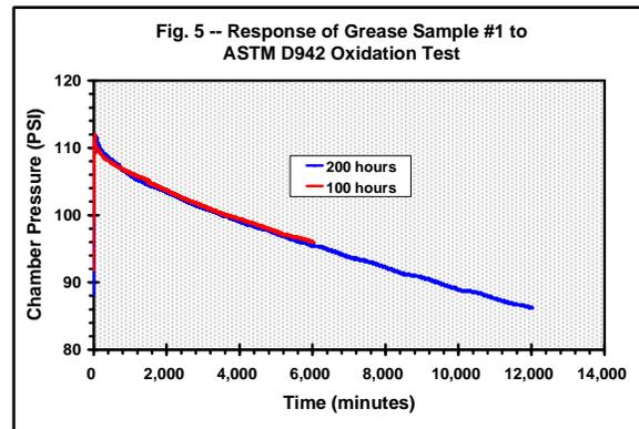
Grease #1 was run at both 100 hours and 200 hours for comparison of both:
