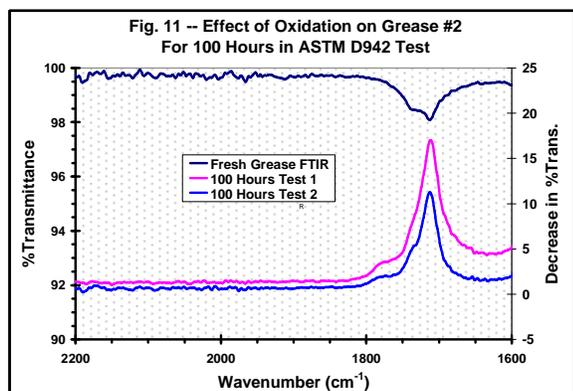
The peaks of Test 1 and Test 2 are both at  $1710\text{ cm}^{-1}$  with reduced Percent Transmittance of 17% and 11% respectively at this wavenumber closely associated with hydrocarbon oxidation.
