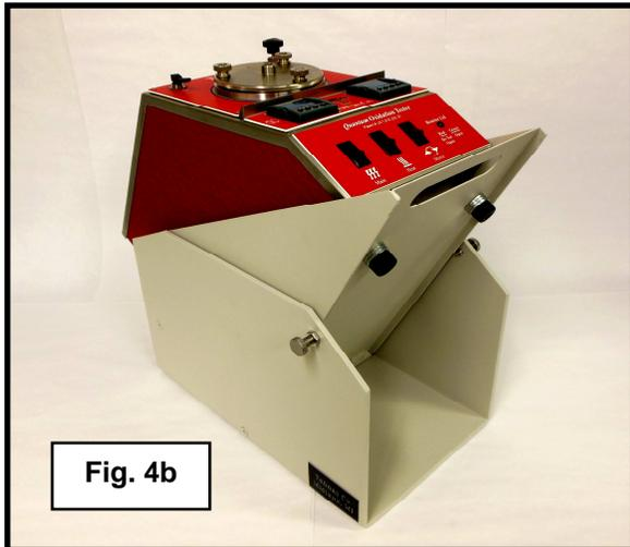
In Fig. 4b, the shelf holding the Quantum is tipped up to the position in which the pressure chamber within the Quantum is vertical and the steel sleeve and rack of grease-containing dishes are installed awaiting sealing the lid and pressuring the closed chamber with oxygen.
