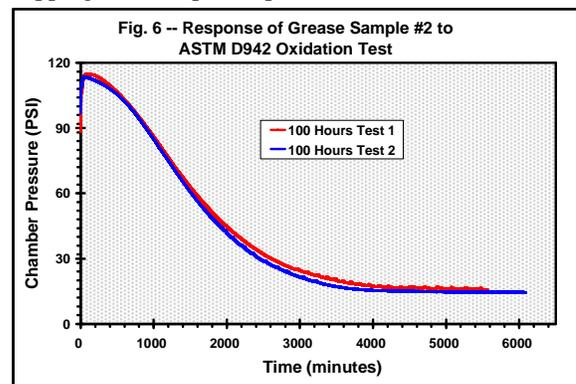
**3.3 Grease #3** – As mentioned earlier, according to the protocol of ASTM Test Method D942, when the oxygen pressure rises to 110 ±2 PSI, the oxygen is carefully released to keep it at this level until oxidation of the grease begins.
