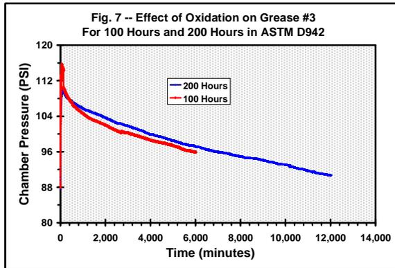
Final oxygen pressures were 96 PSI after 100 hours for Test 1 and 91 PSI after 200 hours for Test 2.
