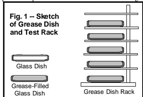
The combined stack of grease-filled dishes are then inserted into a cylindrical pressure chamber and exposed to oxygen of not less than 99.5% purity at an initial pressure of 100 pounds per square inch (PSI = 690 kPa) and room temperature which is then increased to 99 ±0.5°C. Under this increased temperature, the oxygen pressure is carefully released to maintain no more than 110 ±2 PSI).
