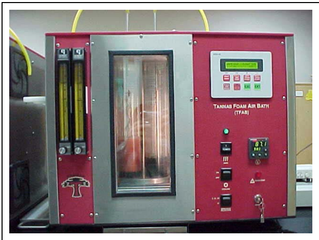
Figure 1 - Air-heated foam test bath used for development of Foamgen ® Test. Two cylinders at a time are rotated by carousel (Figure 2) in front of window for view of foaming behavior.
