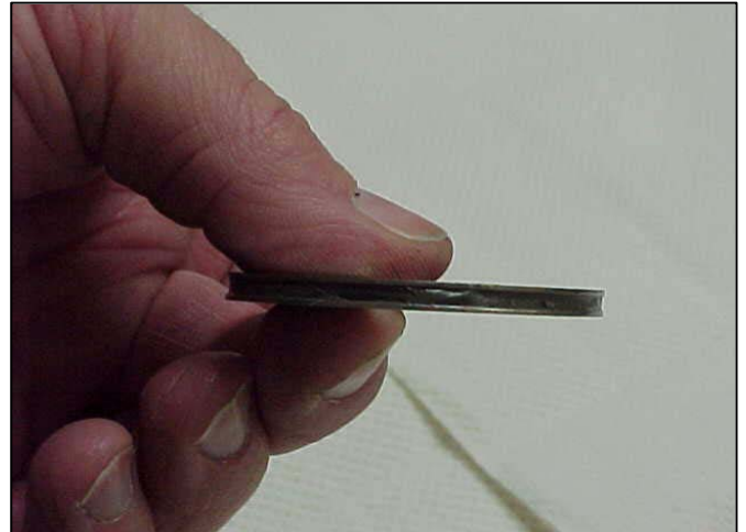
Figure 2 - Picture of a 'button sandwich' of elastomer gasketing material between two precisely spaced steel disks.
