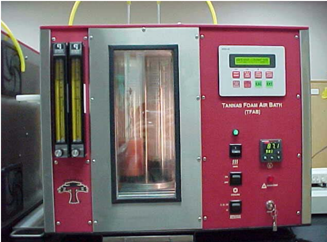
Figure 4 - Air-heated foam test bath used. Two cylinders at a time are rotated by carousel (Figure 5) in front of window for view of foaming behavior.
