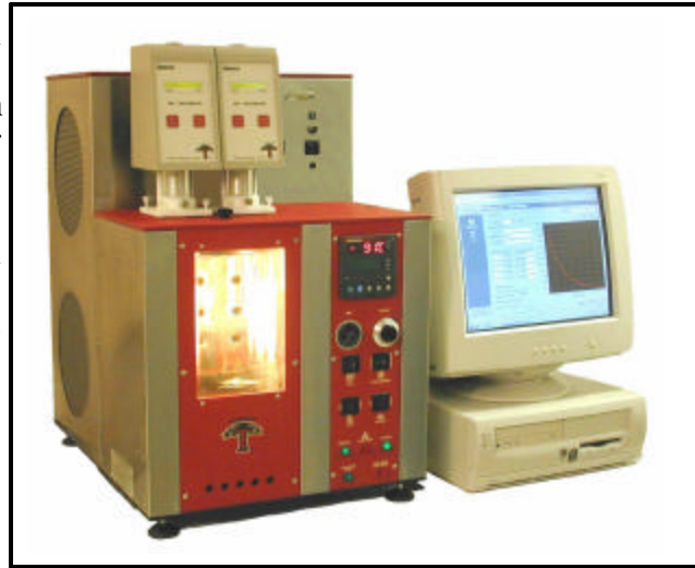
Figure 1 - Tannas PlusTwo bath and viscometer heads with computer and programs
