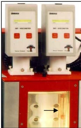
Fig. 2 – TAV-3 viscometer heads set up for SBT analysis on a liquid bath.
