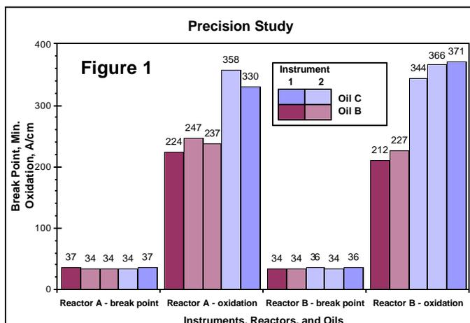
The data show that repeatability within and between instruments is good; particularly considering the difficulty normally associated with reproducing oxidation levels in most instruments.
