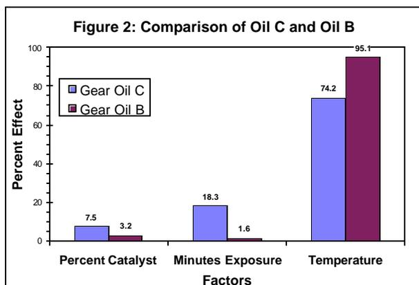
The Taguchi L-4 test clearly shows that exposure temperature has the greatest influence on the oxidation levels of both oils under this Taguchi protocol.
